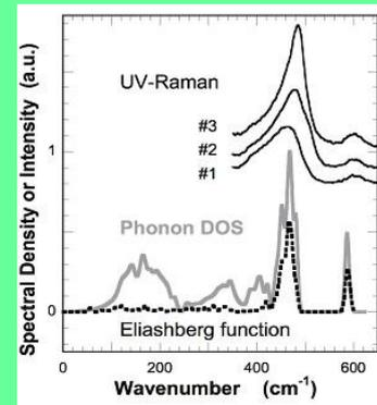
Fig: Experimental Raman spectrum and theoretical phonon density of states and Eliashberg function.
